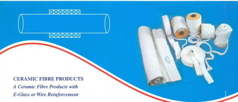
Ceramic Yarns are manufactured from refractory oxides having composition of Alumina, Silica and some special additives. Depending on the use . basic Yarn is reinforced with "E" Glass filament, SS Wire or inconel wire. These Yarn are then finally braided to make rope or woven to make cloth, tape and sleeves.
